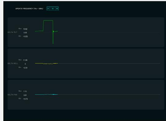
**Hint:** In the left figure below, there is no overshoot in the positive direction, but there is in the negative direction. Increase the TILT value to eliminate the overshoot in both direction as shown in the figure on the right.
